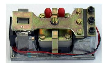
This instruction explains the procedure to replace the diaphragms of sample gas pumps (PN 42716569) used in the X-STREAM series gas analyzers.
